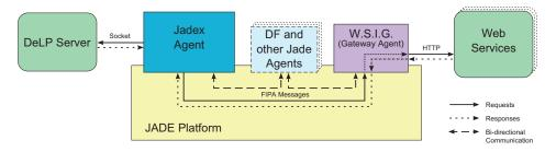
Figure 1: The integration architecture.
